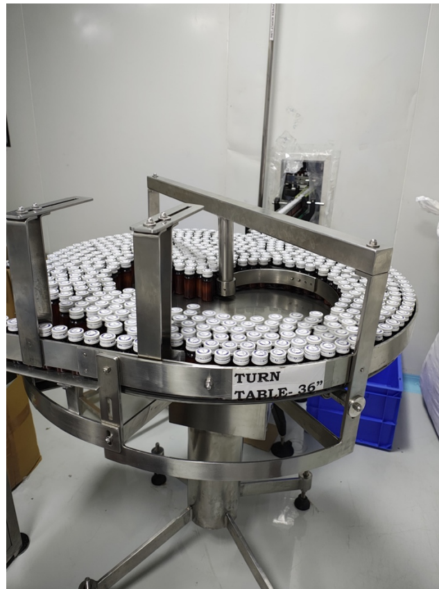
SS TURNTABLE WITH VARIABLE FREQUENCY DRIVE UNIT
