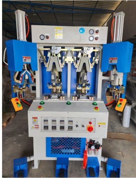
Example of a Pneumatic Counter Molding Machine used in footwear industry
