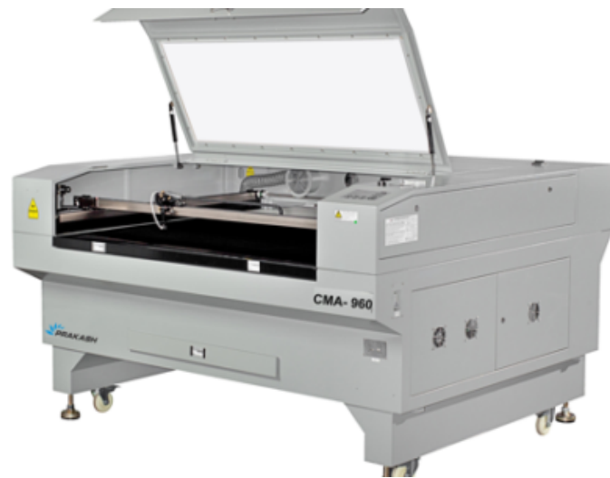
Example of a Laser Cutter used in the footwear industry
